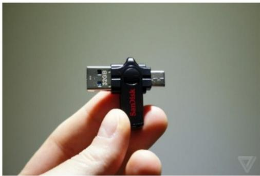
**USB flash drives:** Another advanced form of flash memory is the USB Flash drive, also known as thumb drives and memory sticks. They are portable or removable devices, it doesn't require a device driver. Due to their small size and ease of use, they have superseded floppy disks and zip disks. These two are now considered as legacy technology.
